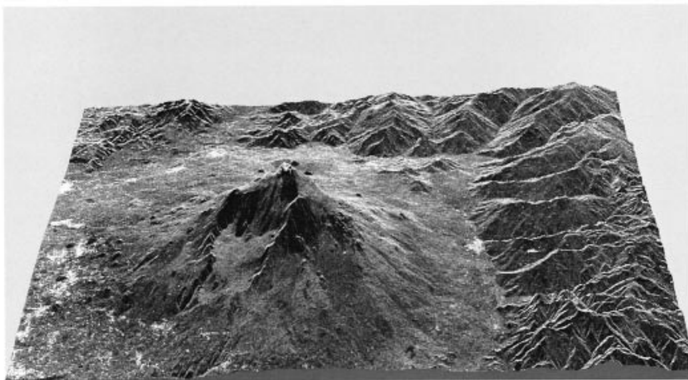
Fig. 11. Dashed area of Fig. 6(b) (perspective view; the grayscale represents the amplitude of the corresponding complex interferogram).
